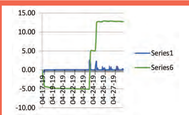
System 2: Graph of Instantaneous & Integrated battery current vs time
