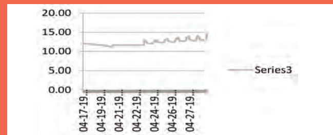
System 1: Graph of Battery voltage during discharge and charging vs time
