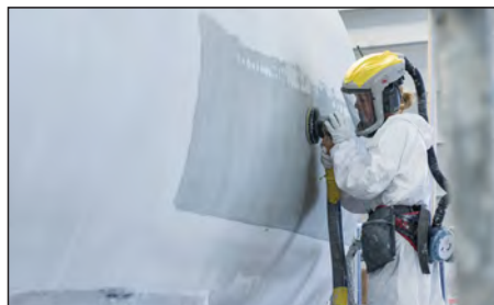
A view of the blade finishing work... Picture Credit: LM Wind Power
