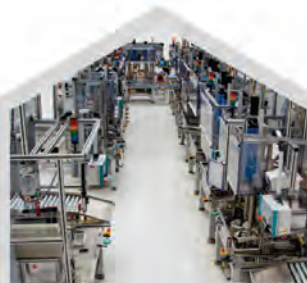
Linear Transfer Assembly Line
