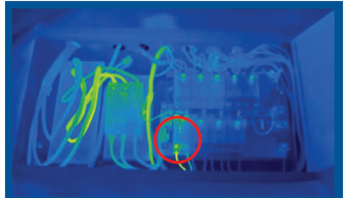
High-pixel camera ( 640 \times 480 pixels) Even when the entire panel is displayed, the heat-generating point is clearly shown due to the high resolution.
