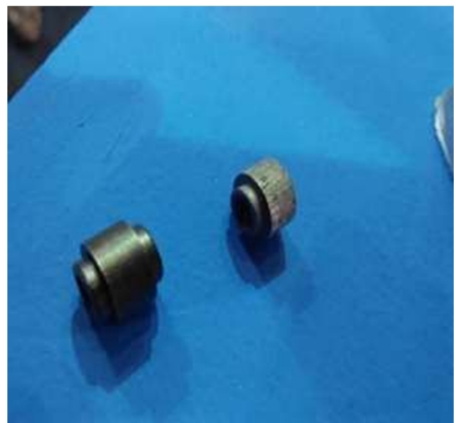
Figure 14. Diamond Wire Beads/Segments
