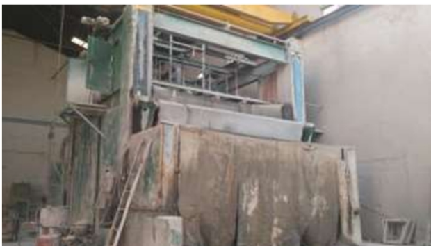
Figure 25. Sawing Blocks using Gangsaw Machine
