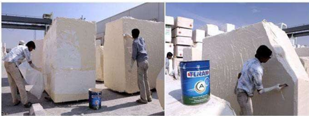
Figure 24. Reinforcement Process of Marble Blocks
