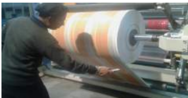
Fig. Unit has designed and provided special type of cutters on shop-floor to the personnel for cutting purpose in order to eliminate cut injuries at the unit.
