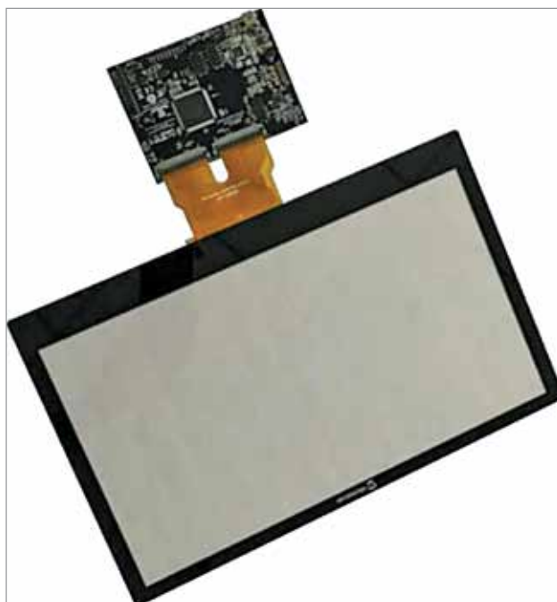
Fig. 4: Microchip's ATEVK-MXT2952T2 evaluation kit contains a dedicated sensor with a flex connector and an electronic control board
