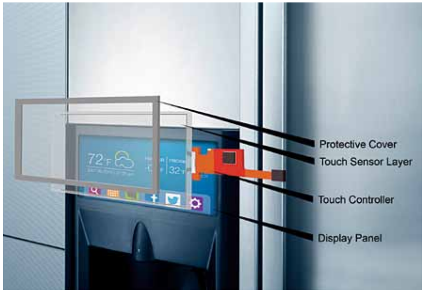
Fig. 2: Behind the touch screen, an array of drive electrodes receives electrodes and the circuitry in the touch IC faithfully detects a user's touch
