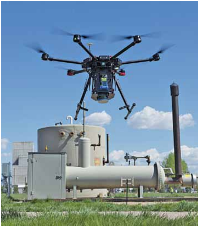
A drone sniffs for methane leaks (Credit: https://news.stanford.edu )
