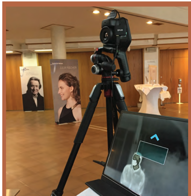
Each screening stations included a FLIR thermal imaging camera with Screen-EST™ mode activated...
