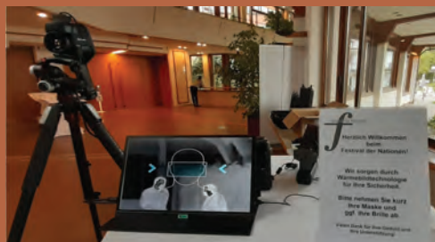
One of three skin temperature screening stations with a FLIR E54-EST camera. Clear instructions helped streamline the temperature measurement process...
