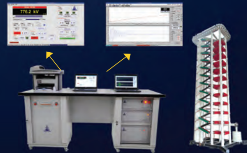
Impulse Voltage Test System
