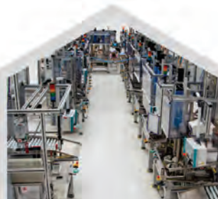
Linear Transfer Assembly Line
