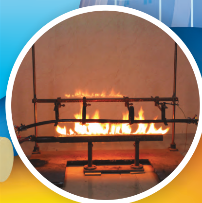
Fire Survival Category CWZ Set Up
